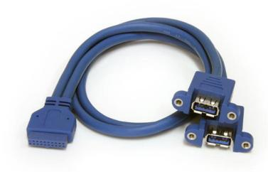
The USB3SPNLAFHD 2-Port USB 3.0 to Panel mount USB cable features a 20-pin USB 3.0 motherboard header connection on one end, breaking off into two separate USB 3.0-A (female) ports on the other end of the cable.
