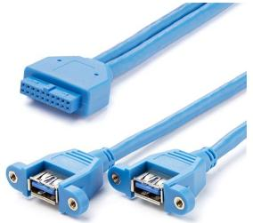
The USB3SPNLAFHD 2-Port USB 3.0 to Panel mount USB cable features a 20-pin USB 3.0 motherboard header connection on one end, breaking off into two separate USB 3.0-A (female) ports on the other end of the cable.
